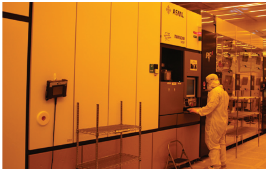
65 nm capable ASML XT:1250
