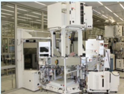
65 nm node metal etch with LAM 2300 Versys
